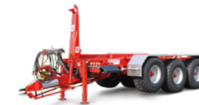
THL 30 (31-34 t total weight, 30 t lifting capacity)
