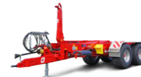
THL 20 (20-24 t total weight, 17-21 t lifting capacity)
