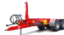
THL 20 (20-24 t total weight, 17-21 t lifting capacity)
