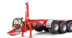
THL 30 (31-34 t total weight, 30 t lifting capacity)
